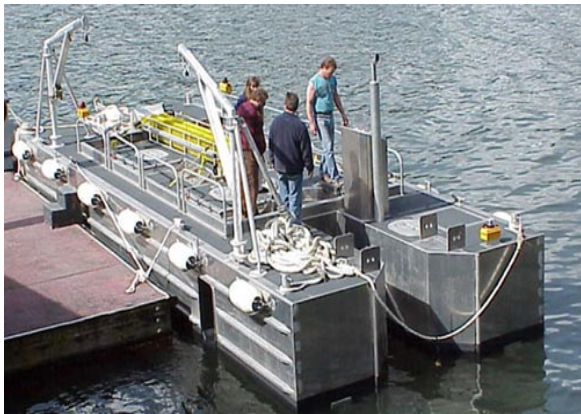
One of the oil-spill response barges stationed in Glacier Bay, Alaska (Photo courtesy of and © ADEC)
