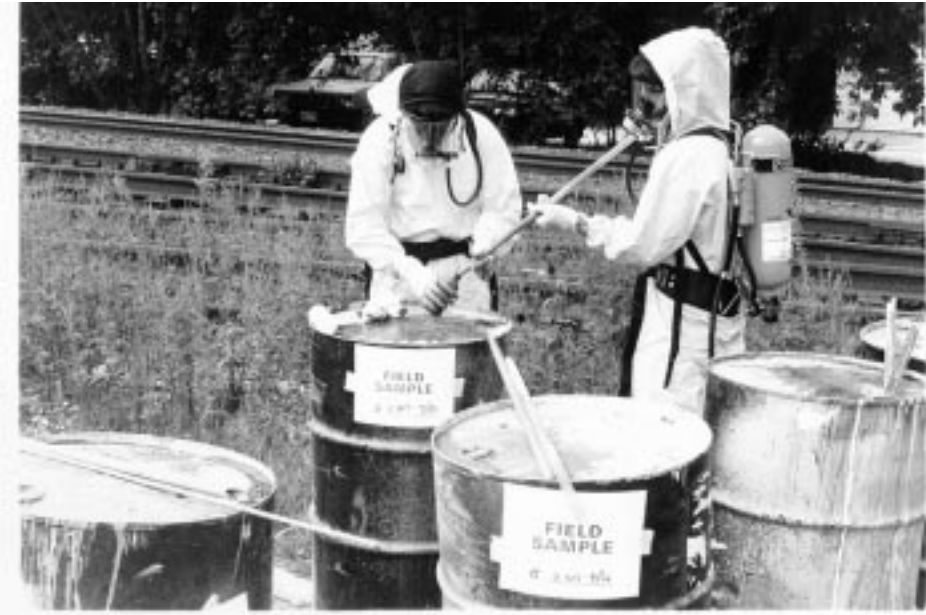
Figure 1 Health Department members of the Hazardous Material Response Team draw samples of the contents of these 55 gallon drums, which were abandoned near a commuter railroad station
