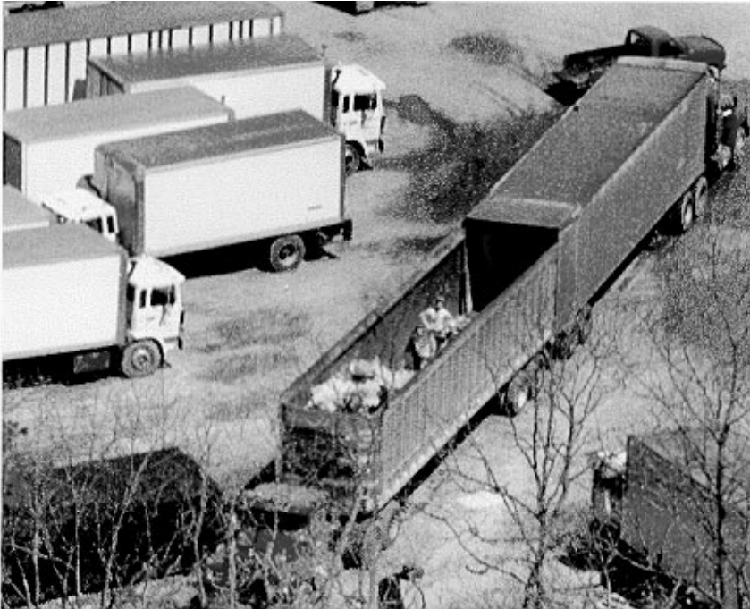
Figure 1 An illegal asbestos storage facility. Note the workers' lack of respirators
